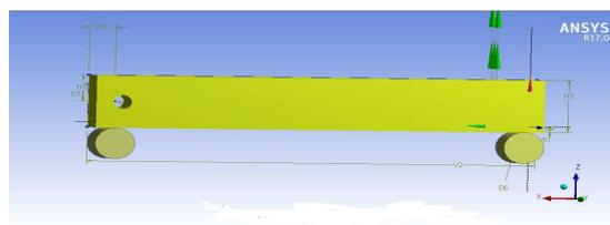
**Figure 6: RC Beam with a Circular Opening near Left Support**
