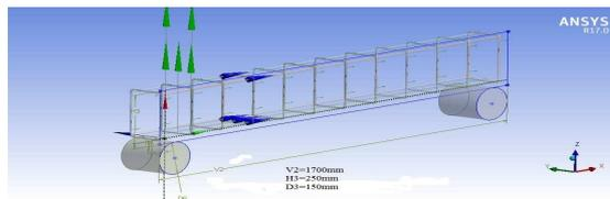
**Figure 2: Reinforcement Detailing of Solid RC Beam Model**
