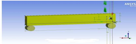
**Figure 10: RC Beam with a Square Opening Near Right Support**
