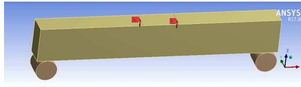
**Figure 4: Four Point Loading-Flexure Test**
