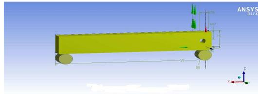
**Figure 7: RC Beam with Circular Opening Near Right Support**
