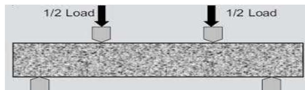
**Figure 3: Four Point Loading-Flexure Test**
