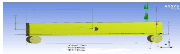
**Figure 5: RC Beam with Central Circular Opening**
