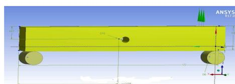
**Figure 11: RC Beam Having 265mm Depth with a Central Circular Opening**
