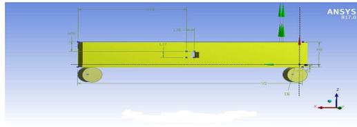
**Figure 8: RC Beam with Central Square Opening**
